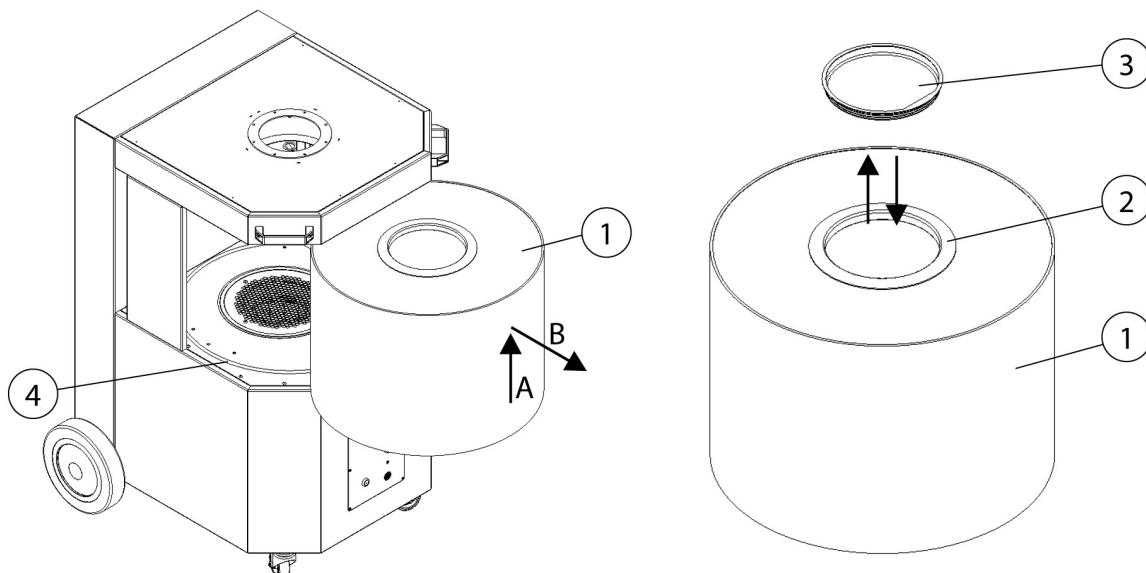
Fig. 12: Filter replacement - Removing the filter element
