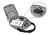
4. Store the pads in the defibrillation pad holder and run the cable through the cable guides.
